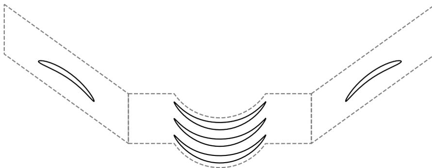
Figure 7: 2D view of the Hanna turbine design with 2 joined rotors (1/16th of the turbine is represented)
