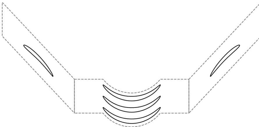
Figure 5: 2D view of the Hanna turbine design (1/16th of the turbine is represented)
