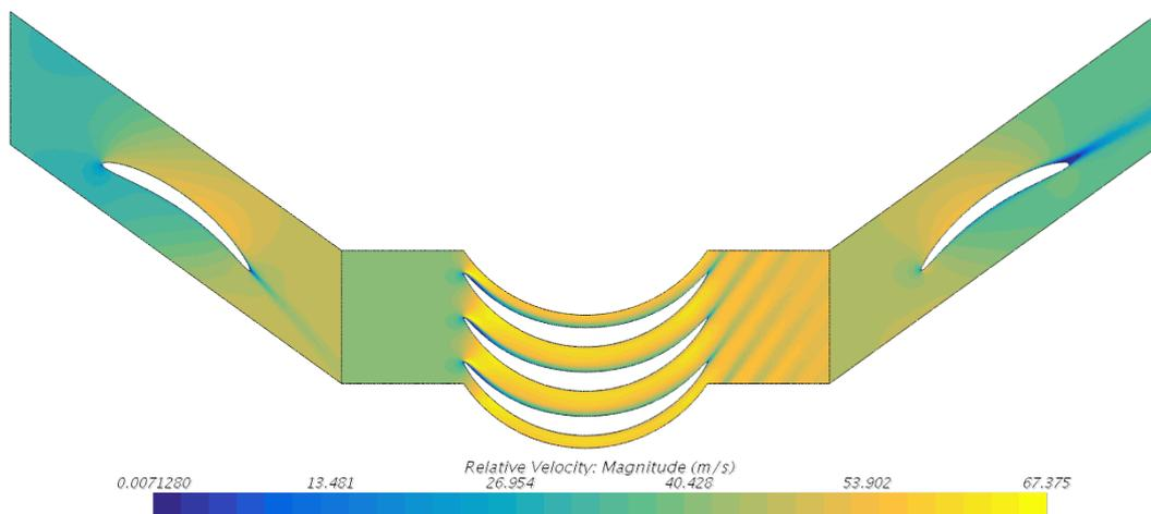
Figure 8: Relative velocity in each row on the Hanna turbine design with 2 joined rotors
