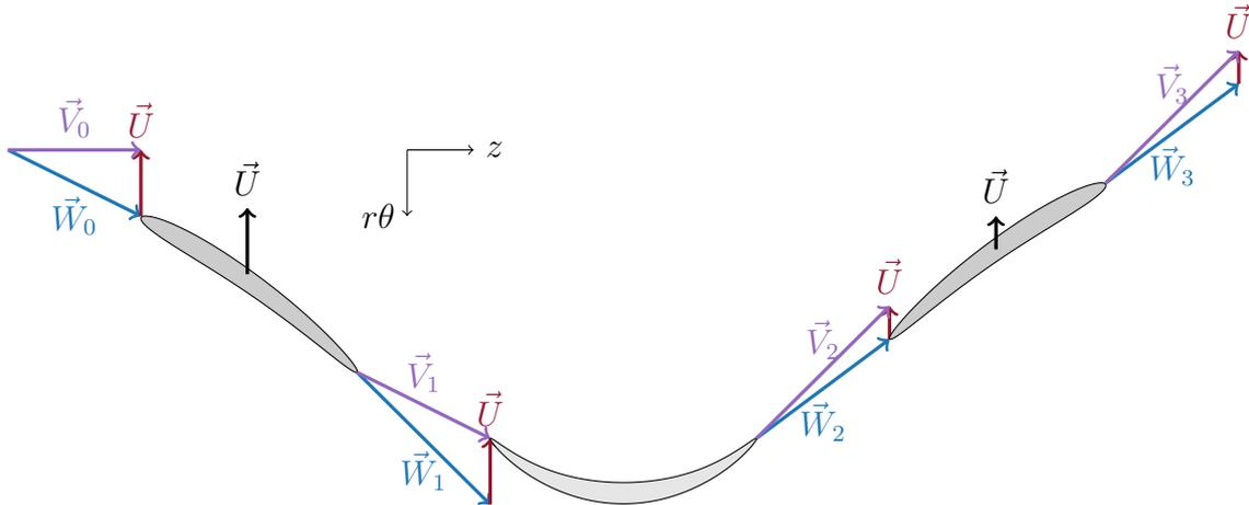
Figure 1: Schematic of the functioning of the Hanna turbine in the blade-to-blade plane
