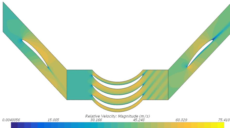
Figure 6: Relative velocity in each row on the Hanna turbine design
