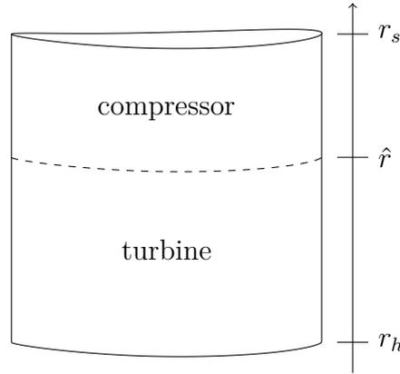
Figure 4: Behavior of a free-wheeling rotor blade
