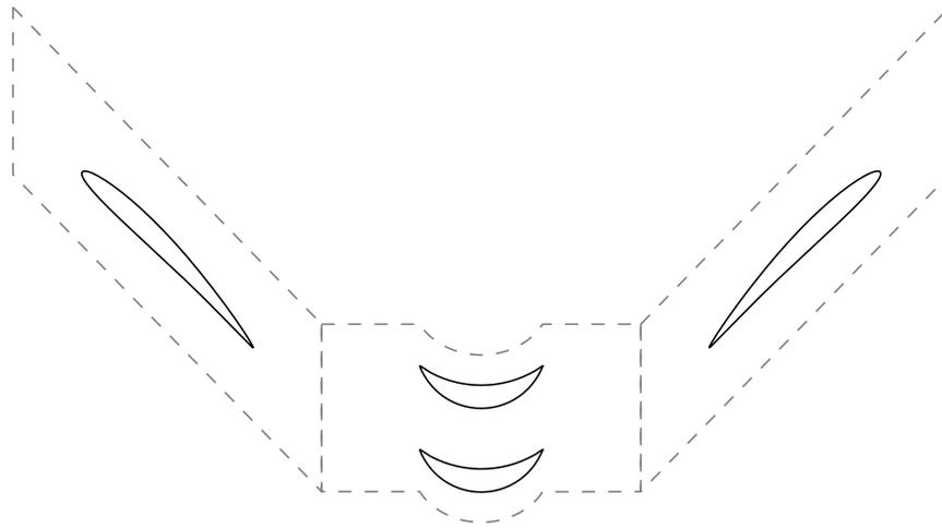
Figure 2: 2D view of the original design of the Hanna turbine (1/18th of the turbine is represented)
