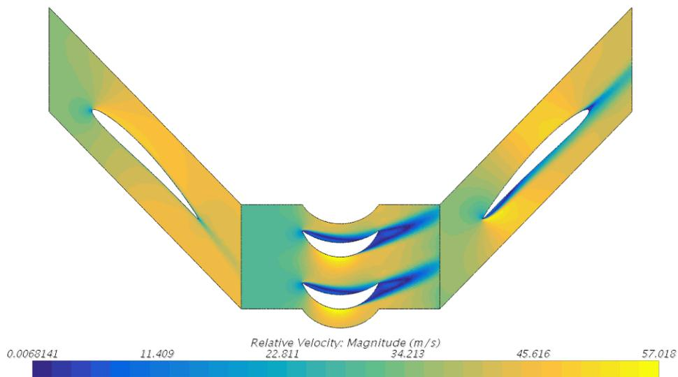
Figure 3: Relative velocity at each row on the original Hanna turbine design, the second rotor on the right moves in the opposite direction of the first rotor
